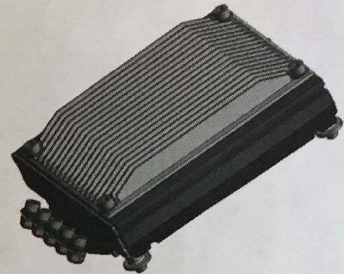
Figure 4.2.1 – Motor Controller and Heat Sink
